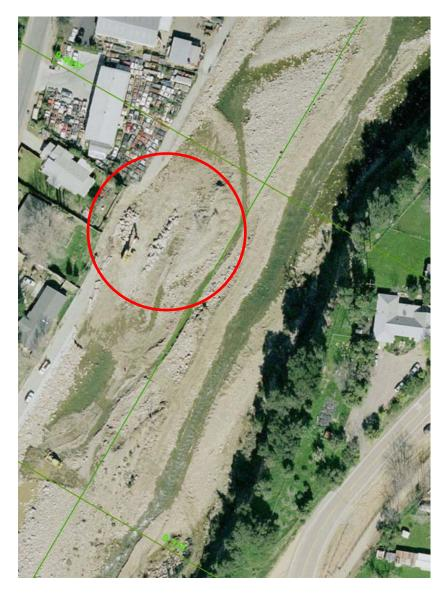
Figure 4.12. Aerial photo taken in February 2005 showing erosion of Live Oak Levee erosion between XC 9.375 and 9.4697.
